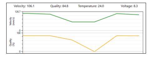
The graph will update automatically, and hence it will easily show if poor signal quality has been achieved. It will be possible to move the MainProbe and check the effect on the graph until Quality improves, or at least is at its maximum for any particular installation.
